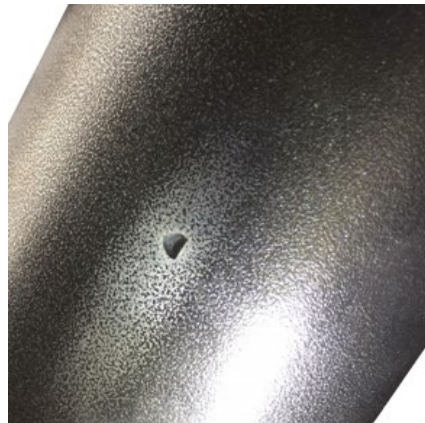
Figure 3: Chafing damage to center spring
