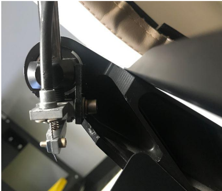
Figure 3.4 Blocking Tab Installed
